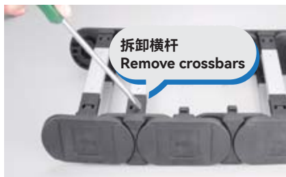
拆卸横杆 Remove crossbars Insert screwdriver into the slot. Using a lever action, release the crossbars
